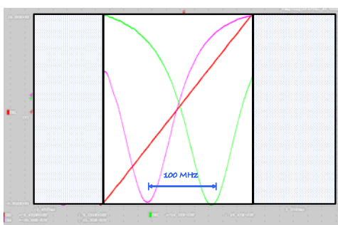
Fig. 3. Experimental spectrum of a 42 cm long spiral resonator.
