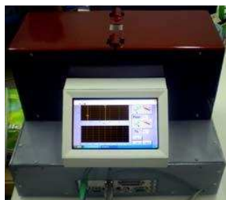
SPR device realised at IMM Institute for liquid and gas measurements in the presence of magnetic field.
